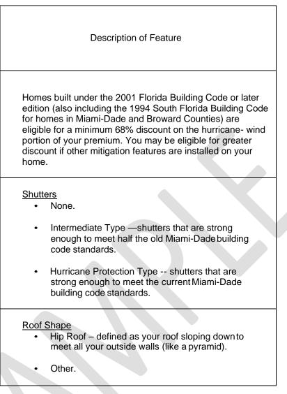
Alternately and regardless of the year of construction, if you meet the minimum fixture and construction requirements of the 2001 Florida Building Code you have the option to reduce your hurricane-wind deductible.
